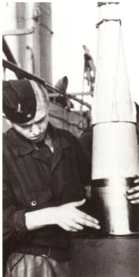
Above: Although many periscopes were made from high quality stainless steel, they still needed a considerable amount of maintenance. The main tube had to be kept greased and lenses often required cleaning and drying out. Condensation was theoretically prevented from forming on the inside by inserting a moisture absorbing cartridge. The active chemical in this was coloured with cobalt chloride, a blue indicator which turned reddish pink when damp. It was then placed on the hot plate of the galley to dry out and could later be reused.
